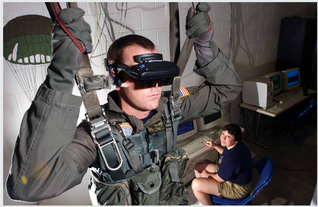
FIGURE 20.16: Virtual Reality (VR) parachute trainer. Students wear the VR glasses while suspended in a parachute harness, and then learn to control their movements through a series of computer-simulated scenarios. The computer receives signals from the student as they pull on the risers that control the parachute. The VR trainer also teaches aircrew personnel how to handle a parachute in different weather conditions and during possible equipment malfunctions.
