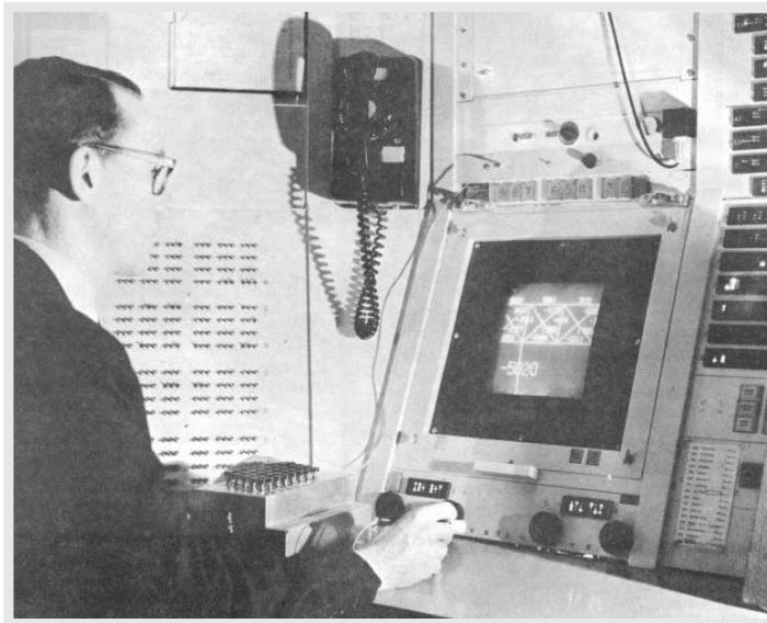
FIGURE 5.12: The TX-2 graphics computer, running Ivan Sutherland's Sketchpad software.
