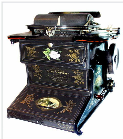
FIGURE 6.2: Typewriter invented by Christopher Latham Sholes, Carlos Glidden and Samuel W. Soule between 1868 and 1873, and manufactured in 1874 by Eliphalet Remington & Sons Co as the ‘Sholes & Glidden Type-Writer’. The colourful flowery decorations may have been intended to appeal to women, who were entering the typist profession.
