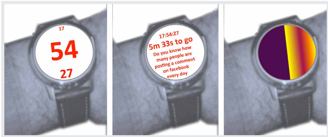
FIGURE 14.2: Design sketches that illustrate ideas for time visualizations in different contexts. Left: for users that run to catch the train; making it easy to see the minutes. Middle: a time visualization for boring lectures and meetings; shows a count down to the end, and some information to engage the user. Right: visualization that gives only a very coarse idea of the time, similar to the information you get from the sun, e.g. for hanging out with friends when time does not matter. With context-awareness, you could create a product that combines all three visualizations and choose the most appropriate one according to the recognized context.
