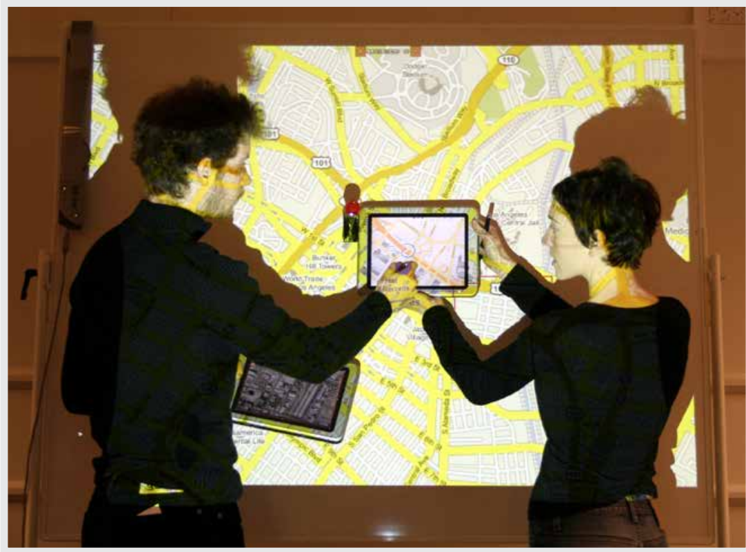
FIGURE 7.3: The ubiquitous graphics system provided a freely movable high-resolution display, that acted as an interactive “magic lens” to reveal detailed information anywhere on the larger display.
