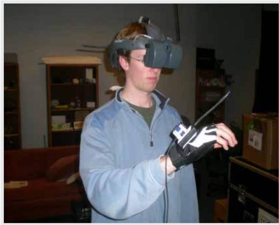
FIGURE 32.2: Using a 3D UI while wearing a head-mounted display. The TV in the background shows the image displayed in the HMD.
