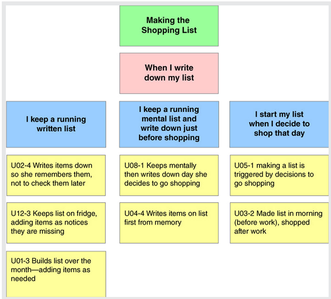
FIGURE 8.7: Portion of an Affinity Diagram. The affinity diagram brings together issues and insights across all customers into a wall-sized, hierarchical diagram to reveal the scope of the problem and the opportunities.
