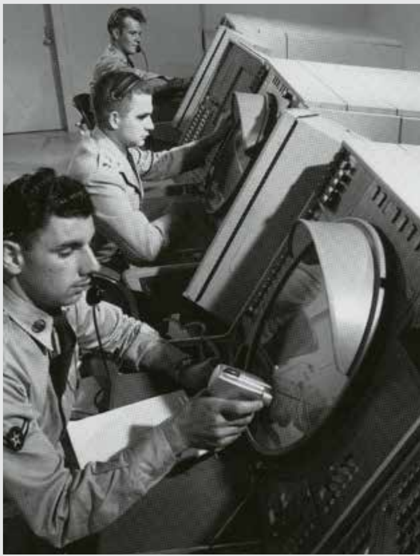
FIGURE 5.10: The SAGE system in use. The SAGE system used light guns as interaction devices.
