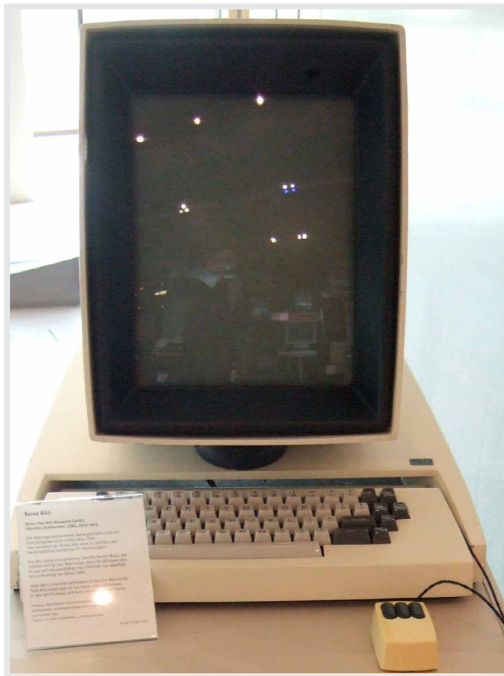
FIGURE 5.25: The Xerox Alto and Apple Lisa, early products in which bitmapped displays allowed pictorial icons to be used as mnemonic cues within the ‘desktop metaphor’
