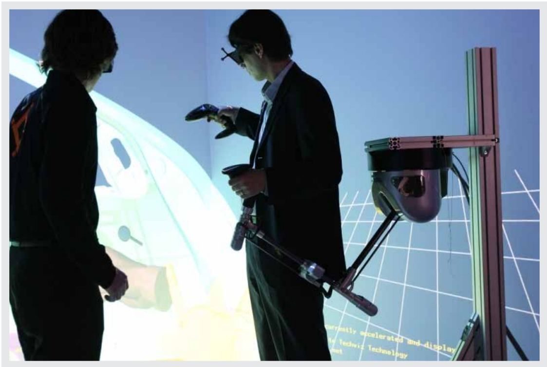
FIGURE 20.15: More sophisticated force-feedback systems (like those manufactured by Haption) can be used to bring rich haptic-reinforcement into virtual environments.
