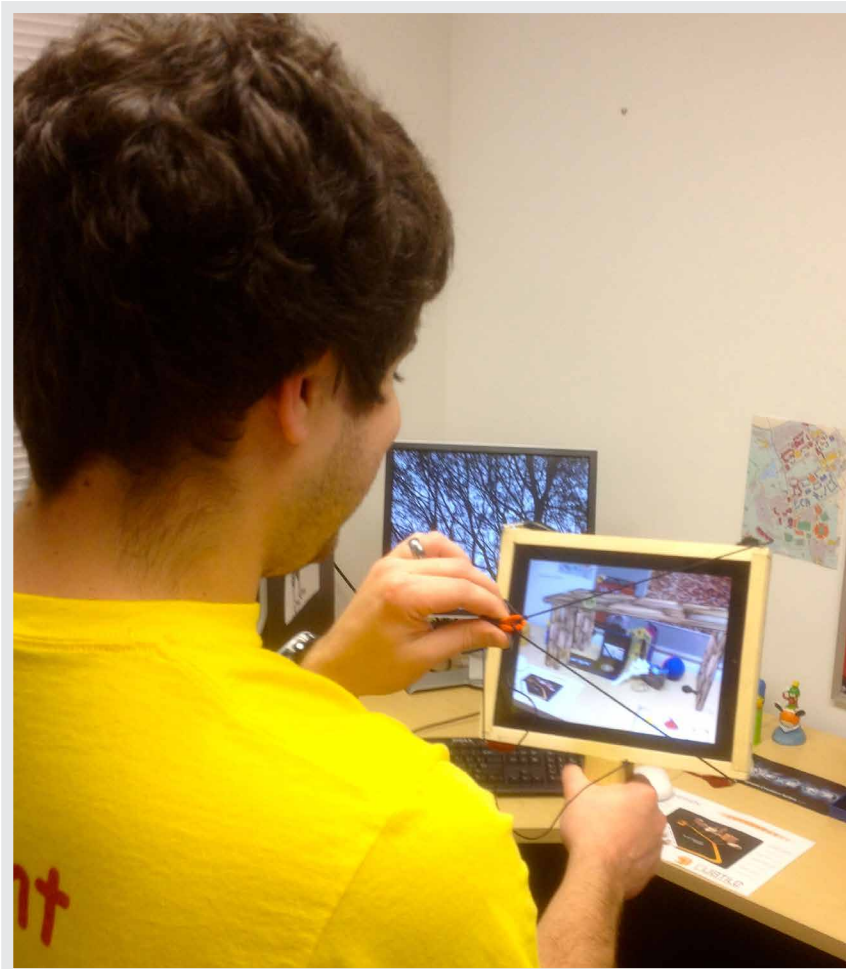
FIGURE 32.3: AR Angry Birds prototype with a physical slingshot and “destruction” of real-world objects—an example of innovation in 3D UI design.
