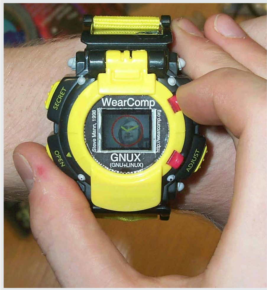
FIGURE 23.19: A wristwatch computer with videoconferencing capability running the videoconferencing application underneath a transparent o'clock, running XF86 under the GNUX (GNU+Linux) operating system. The computer, being general-purpose in nature, rather than task-specific (e.g. beyond merely keeping time, etc.) made this device fit what we typically mean by “wearable computer” (i.e. something that the wearer can reconfigure, program, etc., while wearing it, as well as something that implements Humanistic Intelligence). The project was completed in 1998. The SECRET function, when selected, conceals the videoconferencing window by turning off the transparency of the o'clock, so that the watch then looks like an ordinary watch (just showing the clock filling the entire 640x480 pixel screen). The OPEN function cancels the SECRET function and opens the videoconferencing session up again. The system streamed live video at 7fps, 640x480, 24 bit color.
