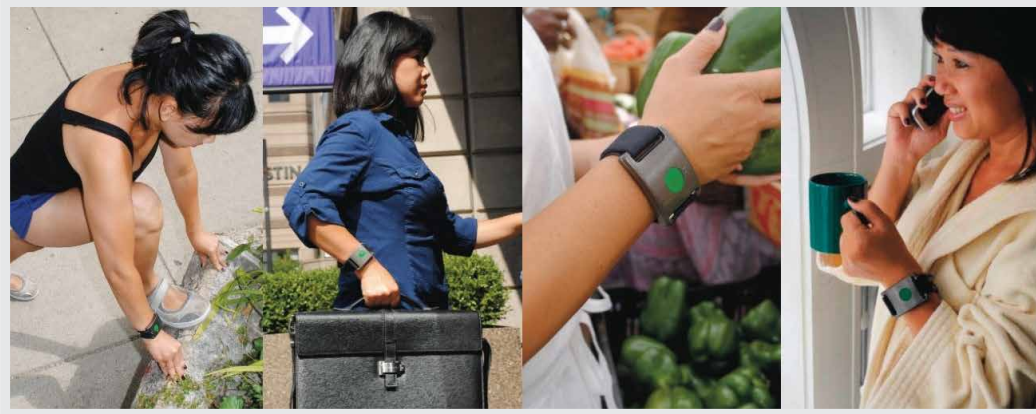
FIGURE 12.8: The bracelet, named Q Sensor, measures skin conductance which in turn is related to emotional arousal - both positive and negative.
