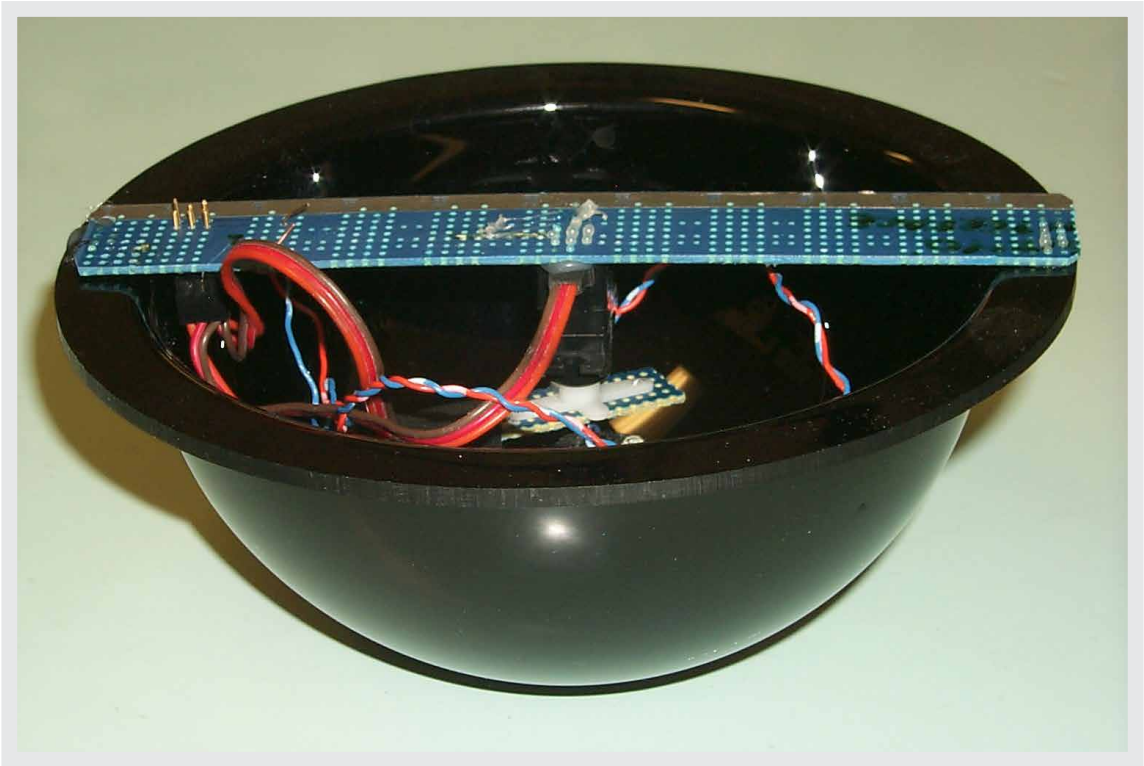
FIGURE 23.6: Closeup of dome pendant showing the laser-based infinite depth-of-focus projector, called an “aremac” (Mann 2001). The laser-based aremac was developed to project onto any 3D surface and does not require any focusing adjustments.
