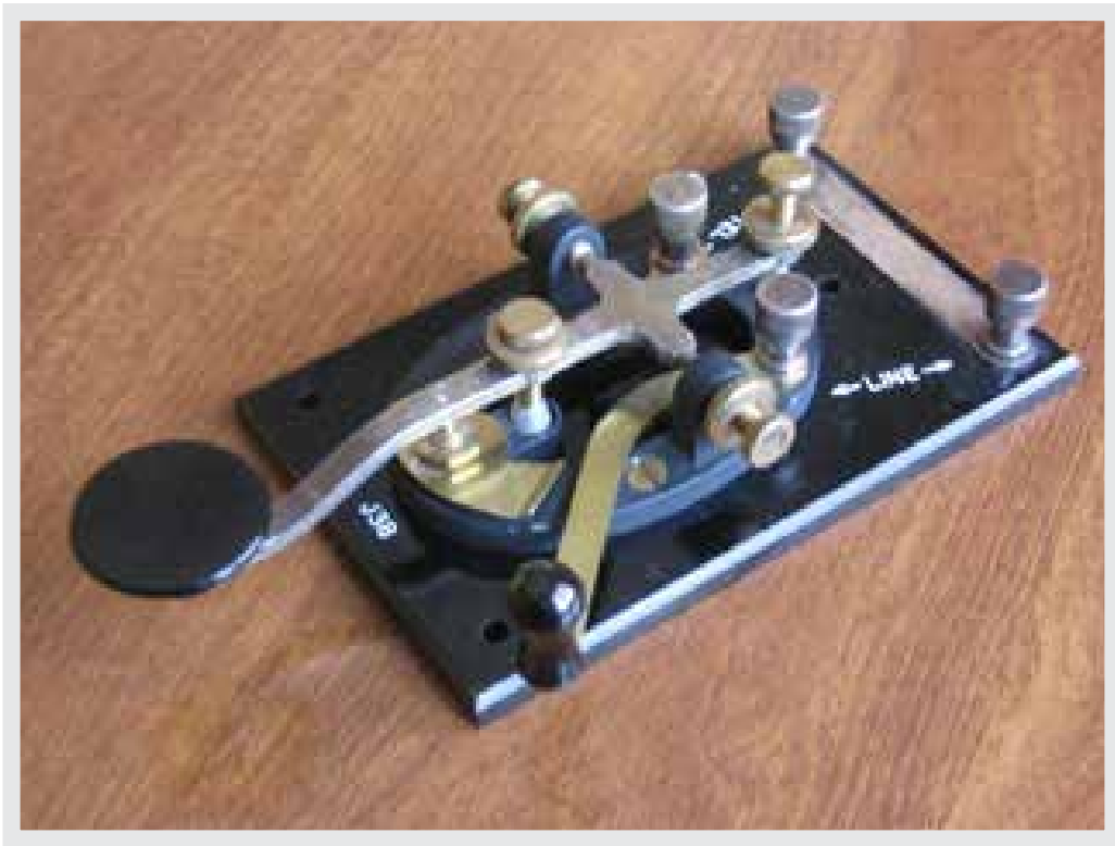
FIGURE 23.22: Original wearable computer input devices were inspired by the telegraph key -- This particular telegraph key is a J38 World War II-era U.S. military model.
