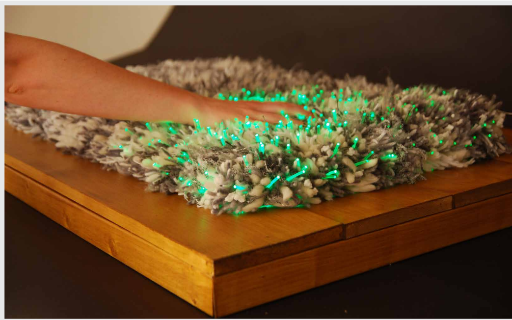
FIGURE 6.31: PeR, Perception Rug, designed by Eva Deckers. PeR is a knotted carpet in which touch sensitivity and optic fibres are integrated. PeR has the ability to perceive and react to perceptive activity of people. PeR can adapt different perceptive behaviours.
