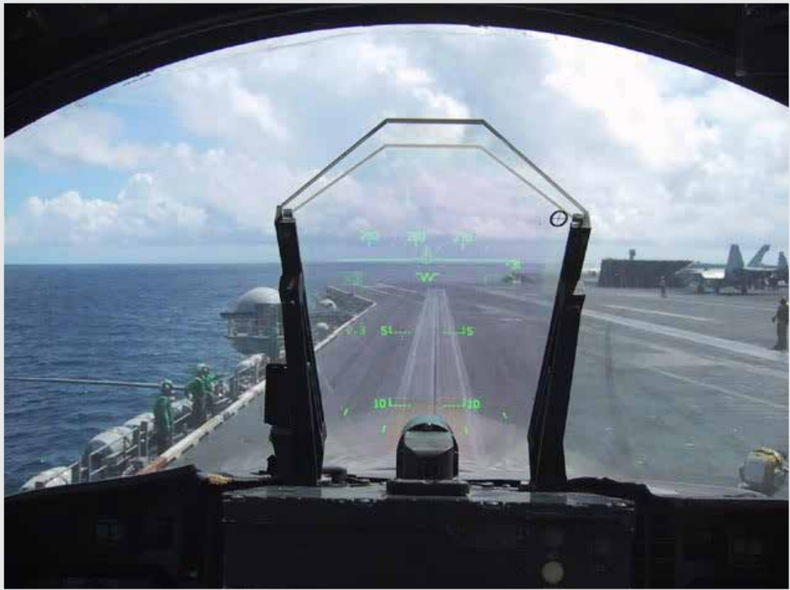
FIGURE 23.2: Photograph of the Head-Up Display taken by a pilot on a McDonnell Douglas F/A-18 Hornet.
