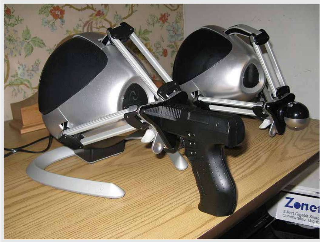
FIGURE 20.13: A Pair of black Novint Falcons sitting on a table, with the Pistol and Ball grip attachments.
