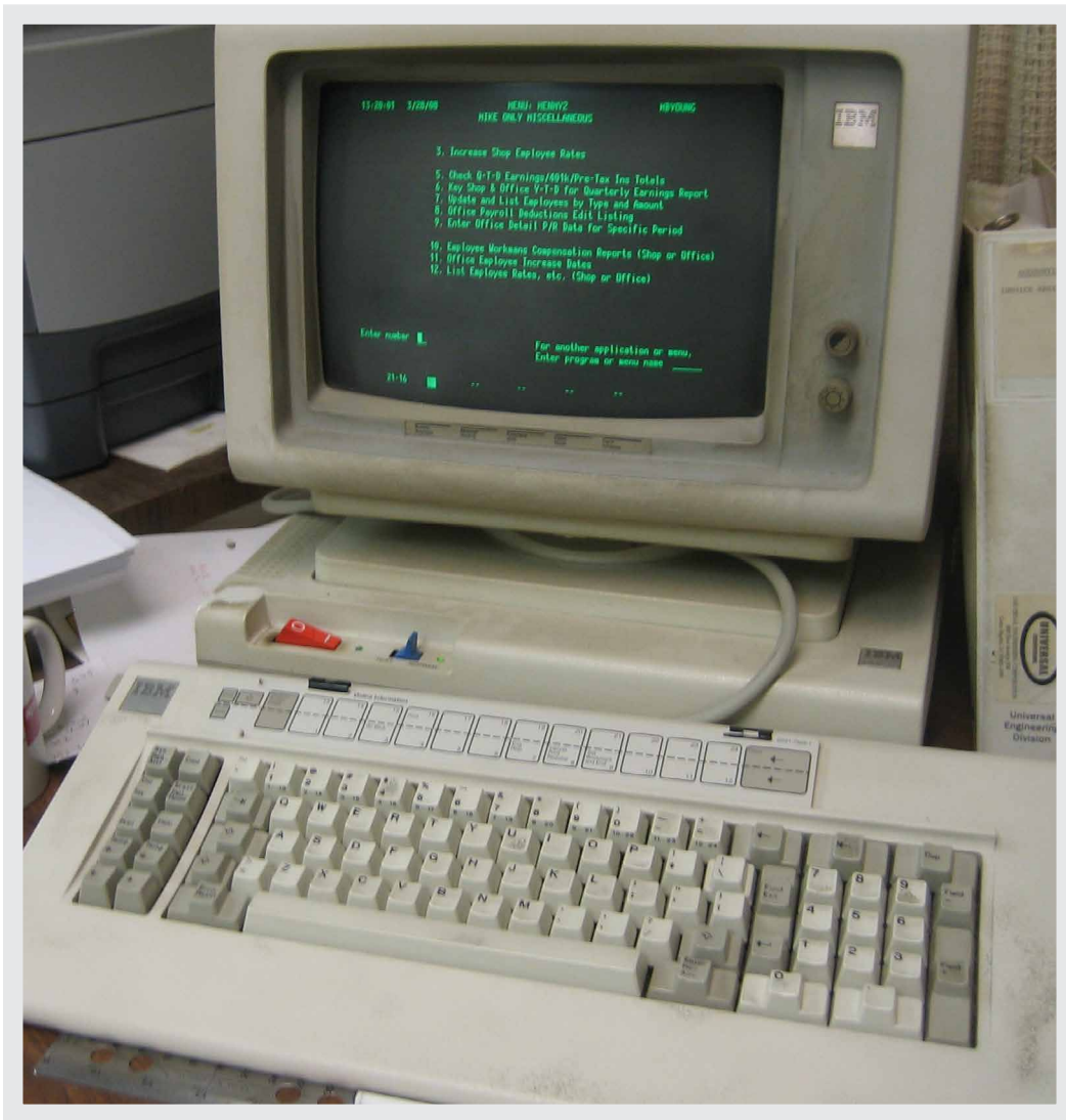
FIGURE 10.2: Terminal interface presenting a fixed menu, where users type a number to indicate a menu selection.
