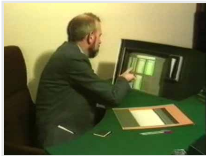
FIGURE 7.7: Direct interaction with the Bifocal Display allows a specific item or area to be dragged into the focus region (from Video 5).
