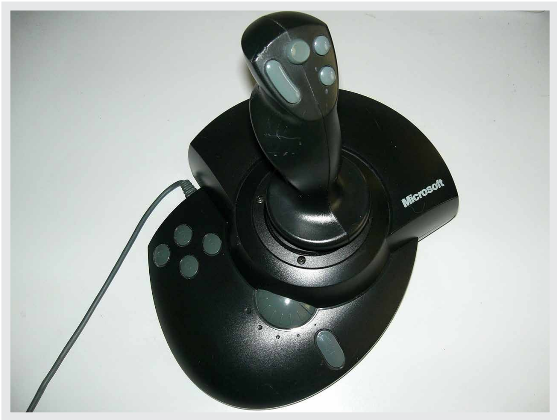
FIGURE 20.14: Video gaming devices can make effective use of force feedback to bring immersive qualities to game-play. These range from vibratory ‘rumble’ pads, to simulate collisions and shockwaves for example, to more physical interactions from a force-feedback joystick like the one pictured here (the Sidewinder Force-feedback Pro from Microsoft) where the hand is controlled and moved, perhaps to suggest resistance from obstacles, or actions like the recoil from shooting a gun.
